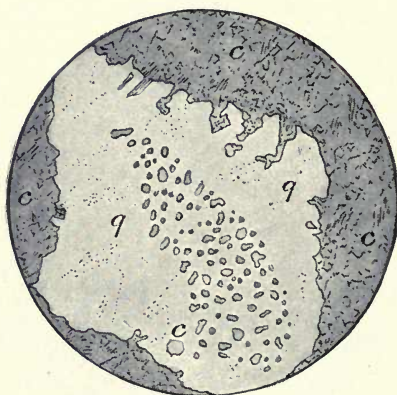
Quartz Grain in Same Section, Partly Replaced by Calcite. q , Quartz; c , calcite with some sericite replacing from outside; also, secondary calcite grains forming on inclined fissure-plane in quartz. Magnified 80 diameters.
